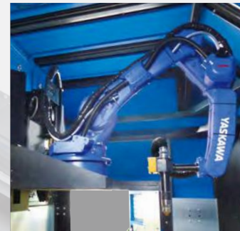
8 AXES ROBOT CELL (6+2) The latest 6 axes MOTOMAN robot, plus the 2 axes MOVING ROBOT BASE expands the plasma torch reach. This improves accuracy of the positioning by avoiding full stretch of robot arms.
