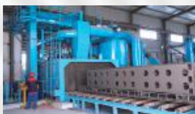
04 Sandblasting and Spraying
